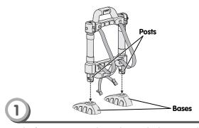
Fit the frame posts into the sockets in the bases. Push to "snap" in place.
